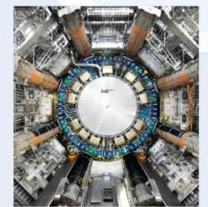
ATLAS is the largest detector ever constructed for a particle collider: 46 m long and 25 m in diameter. Its construction pushed the limits of existing technology.
